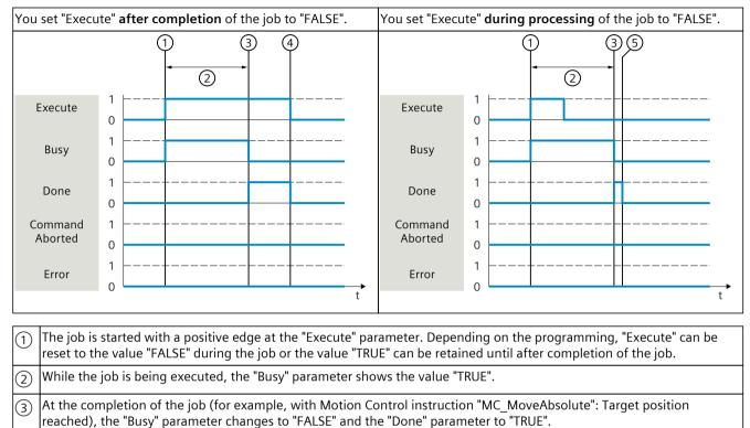
As long as the "Execute" parameter retains the value "TRUE" after completion of the job, the "Done" parameter also retains the value "TRUE".
