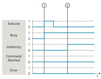
The job is started with a positive edge at the "Execute" parameter. Depending on the programming, "Execute" can be reset to the "FALSE" value before or after the parameterized velocity has been reached. While the job is being executed, the parameter "Busy" shows the value "TRUE".
