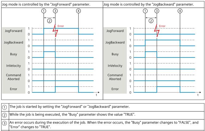
(4) When the "JogForward" or "JogBackward" is reset to the value "FALSE", the "Error" parameter likewise changes to "FALSE".
