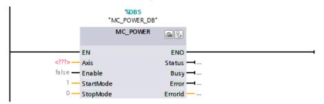
The instance data block is automatically created under "Program Blocks > System Blocks > Program Resources".
